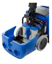
The onboard battery charger gives quick access to charging when needed.
